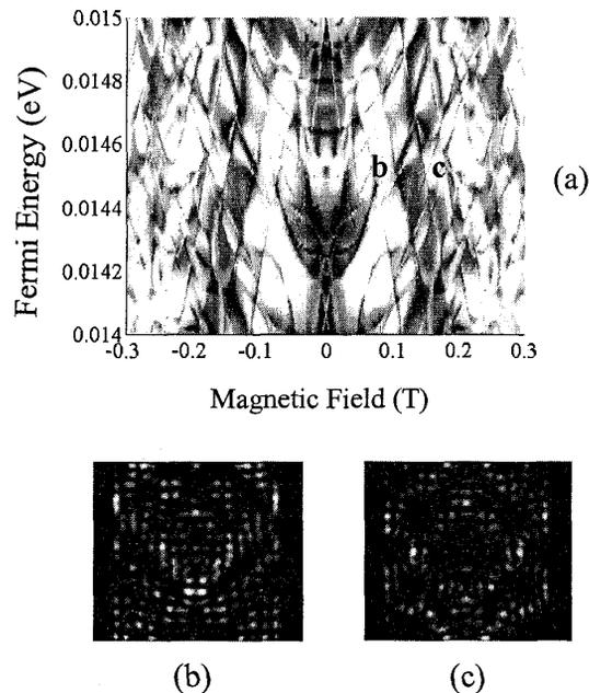
Fig. 3. (a) Conductance as a function of magnetic field and Fermi Energy for a  $0.40 \mu\text{m}$  square dot. (b) Wave function corresponding to point b in (a),  $E_F = 0.145 \text{ eV}$ ,  $B = 0.074 \text{ T}$ . (c) Wave function corresponding to point c in (a),  $E_F = 0.145 \text{ eV}$ ,  $B = 0.182 \text{ T}$ .
