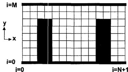
Fig. 1. The geometry of the quantum dot, and quantum point contacts, that are considered in this study. The grid represents the underlying mesh on which the calculations are performed, though in practice the mesh is much finer.
