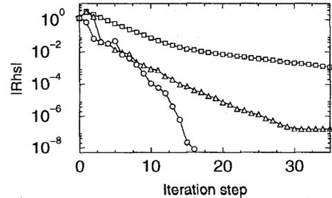
Figure 2: Convergence using Broyden's algorithm (o), a simple mixing method ( $\square$ ) and the Anderson mean value extrapolation method ( $\Delta$ ).
