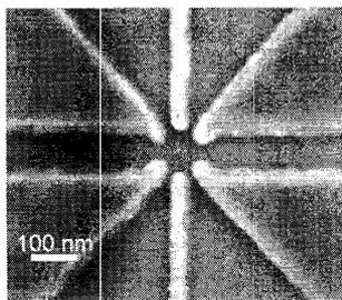
Figure 3: Top view of the Ti/Al gate structure of the SiGe heterostructure SET. Courtesy PSI Villigen.
