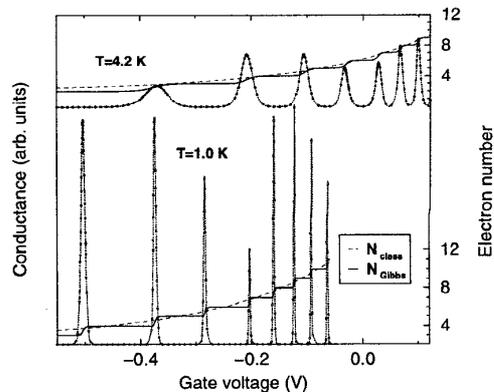
Figure 4: Conductance oscillations and charging of the SET-QD as a function of a plunger gate voltage at two different temperatures. The curves are given an offset for clarity.
