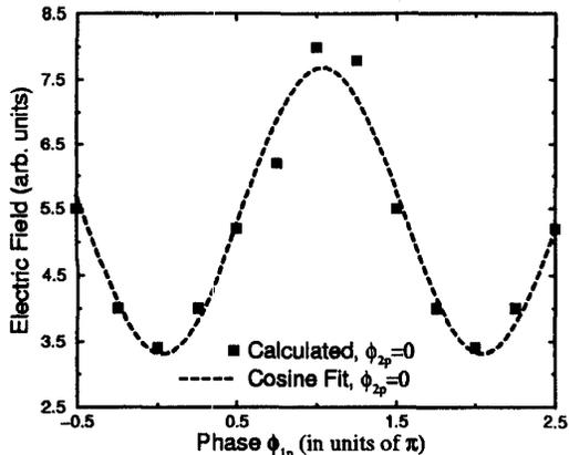
Figure 3: Amplitude of the emitted electric field versus phase  $\phi_{1p}$  (full circles). Dashed line is a cosine fit to the data points.
