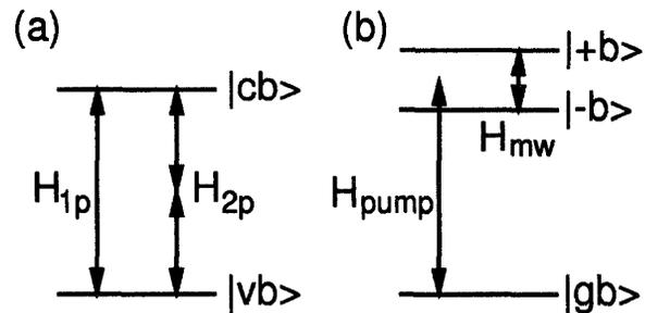
Figure 1: Schematic representation of two coherent control schemes: (a) traditional scheme using interference between single- and multi-photon absorption; (b) a coherent control scheme based on a three-level system. Horizontal bars and vertical arrows indicate electronic bands and light fields, respectively.
