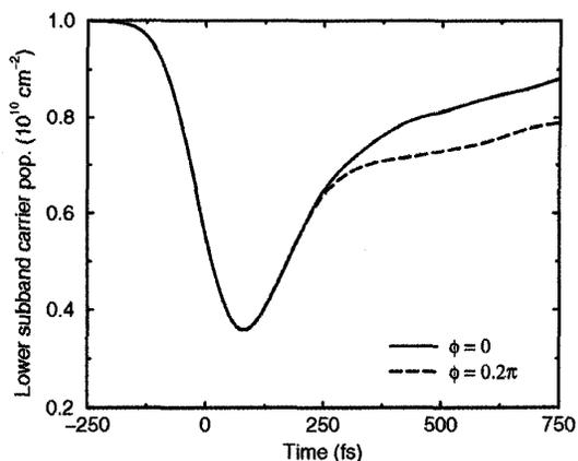
Figure 4: Carrier density in the ground subband  $|g_b\rangle$  versus time. Time zero marks the arrival of the peak of the pump pulse.  $\phi$  denotes the phase of the mw field (relative to the time of arrival of the pump pulse).
