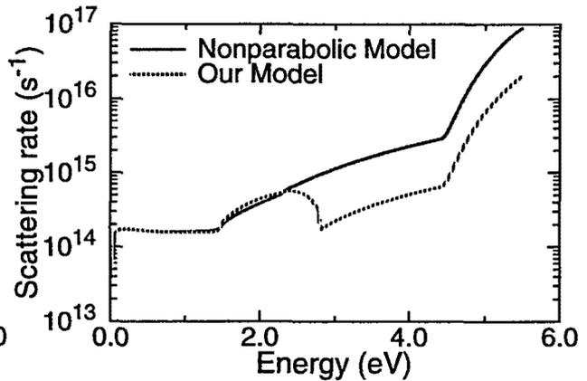
Fig. 2. The electron total scattering rate in the gamma valley for the simple infinite valley nonparabolic model, and our approach.
