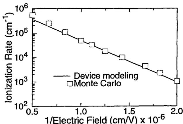
Fig. 5. Impact ionization rate for electrons in ZnS as a function of the inverse applied electric field.
