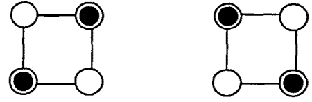
Figure 2. Antipodal alignment of electrons due to Coulombic repulsion. The ground state is highly bistable.
