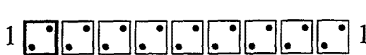
Figure 3. A binary wire. Dot radius on each site is proportional to the actual calculated charge density on that site. Data is transmitted from one end of the wire to the other.
