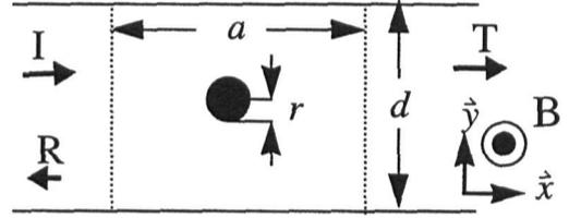
Figure 2. Schematic geometry of a quantum channel with one antidot as a single scatterer in a perpendicular magnetic field.
