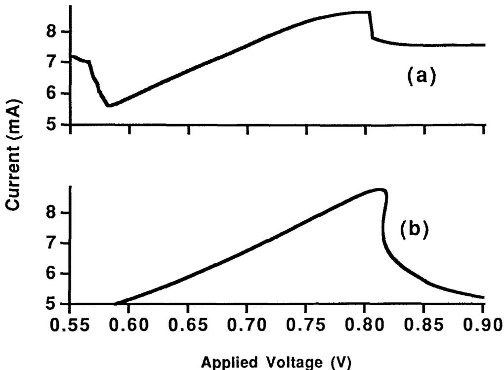
Fig. 2 - Comparison of the experimental phonon-assisted tunneling current versus dielectric continuum model prediction. (a) Expanded view of the experimental current-voltage curve of Fig. 1, focusing on the phonon-assisted tunneling region. (b) Calculated excess current.
