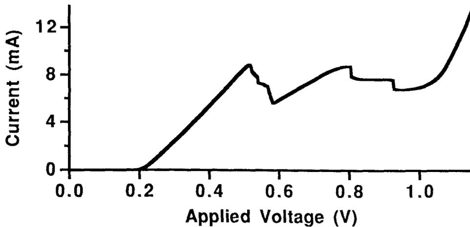
Fig. 1 - Experimental current-voltage curve in the forward bias direction, i.e. the 33 Å barrier as the emitter barrier.
