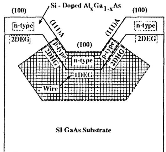
Figure 1: Schematic diagram of the model corrugated  $GaAs/AlGaAs$  heterojunction system.
