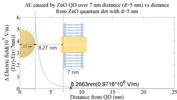
Fig. 2. Electric field produced from the spontaneous polarization of a ZnO quantum dot (diameter=5 nm) versus the distance from the quantum dot. The minimum distance required to switch an ion channel (8.27 nm) is indicated.
