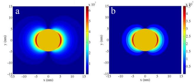
Fig. 3. Electric field due to spontaneous polarization of a 5-nm ZnO quantum dot in water (a) and in electrolyte (b).
