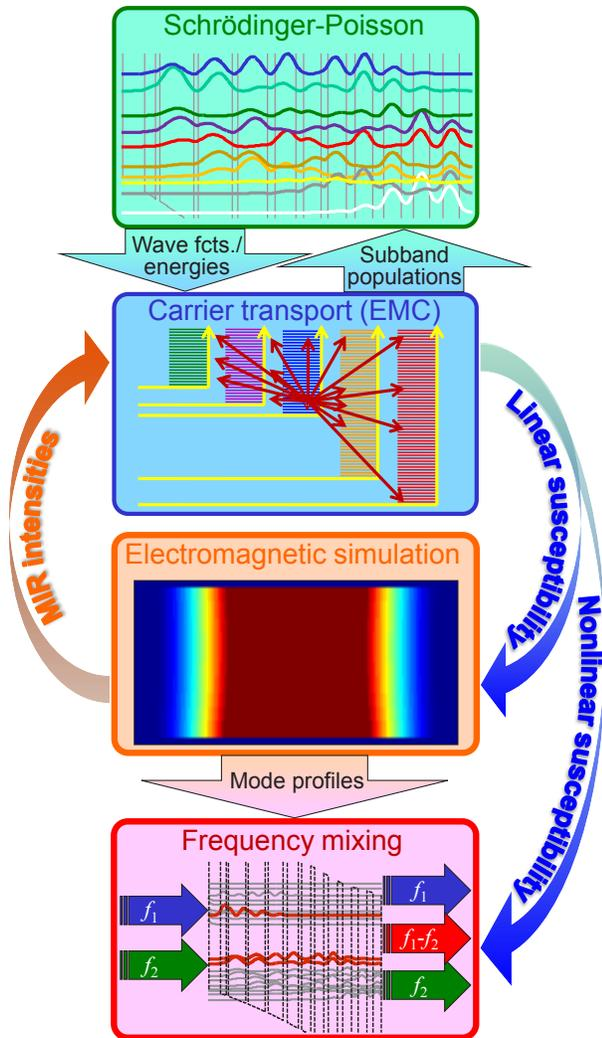
Fig. 1. Schematic illustration of a multi-domain simulation approach for QCL frequency conversion structures.
