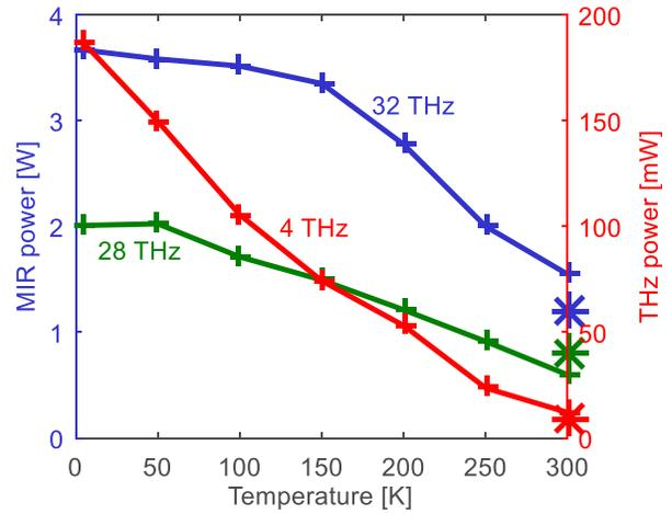
Fig. 2. Simulated MIR and THz powers vs. temperature (solid lines), and available experimental data (asterisks).
