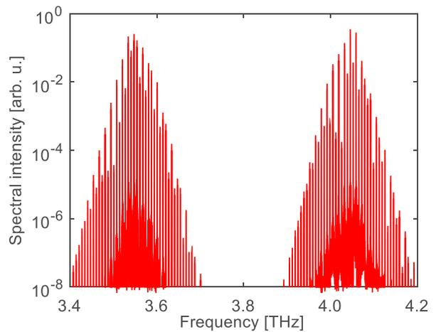
Fig. 4. Simulated optical power spectrum of the QCL frequency comb source in [4].
