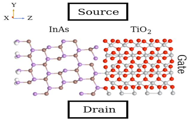
Fig. 2 .InAs/TiO<sub>2</sub> (rutile crystal phase) interface. This structure was structurally relaxed with LDA DFT
