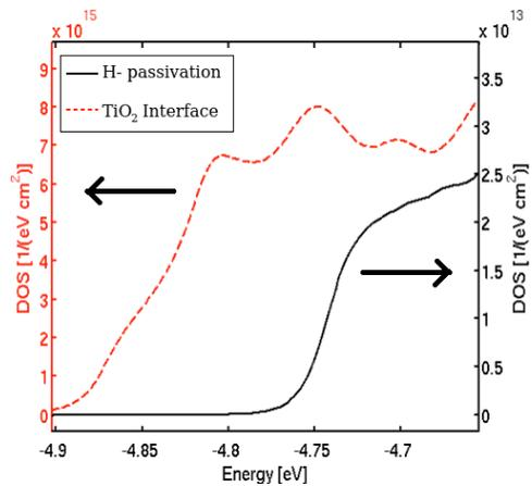
Fig. 6. Density of states comparison of InAs/TiO<sub>2</sub> with H-terminated UTB.
