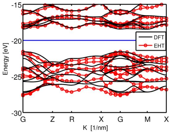
Fig. 3. Example fitting of EHT parameters to DFT Targets for rutile phase of bulk TiO<sub>2</sub>
