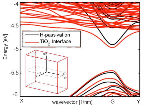
Fig. 4. Band structure comparison of InAs/TiO<sub>2</sub> with H-terminated UTB. Inset: Interface coordinate system and Brillouin zone
