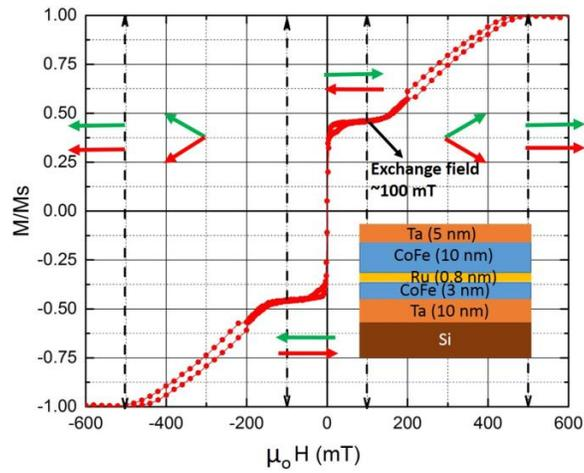
Figure 1: M-H curve for the exchange coupled stack (Green arrow: Magnetization of top layer, Red arrow: Magnetization of bottom layer), stack geometry shown in inset.
