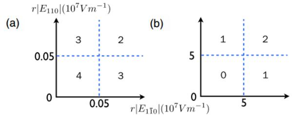
Fig. 4. Quantized conductance (units of  $e^2/h$ ) in TCIs in the (a) thick ( $>20$  nm) and (b) thin film (5-10 nm) limit.
