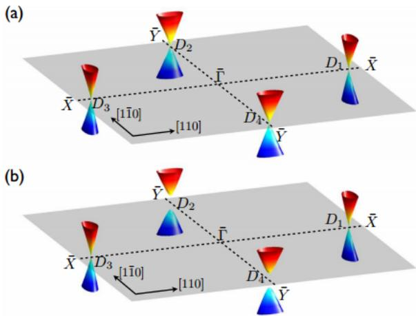
Fig. 2. (a) 2D Brillouin zone along the (001) surface. Gapless surface states emerge on either side of  $\bar{X}$  and  $\bar{Y}$ . (b) Strain in the  $(111)$ -direction opens a gap in Dirac cones  $D_2$  and  $D_4$ , about  $\bar{Y}$ .
