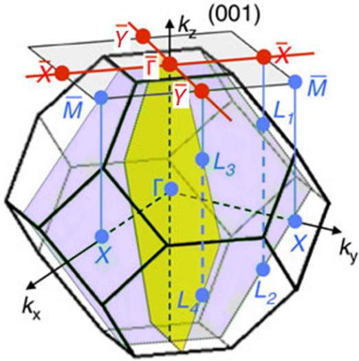
Fig. 1. Rocksalt lattice structure and 3D Brillouin zone of  $\text{Pb}_{1-x}\text{Sn}_x\text{Te}$ . Adapted from [4].
