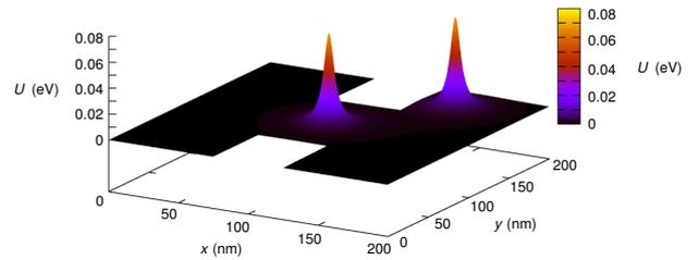
Fig. 4. Graphene constriction, in the presence of a potential given by the sum of two Lorentzian functions with half-width at half-maximum 4 nm and peak height 70 meV.
