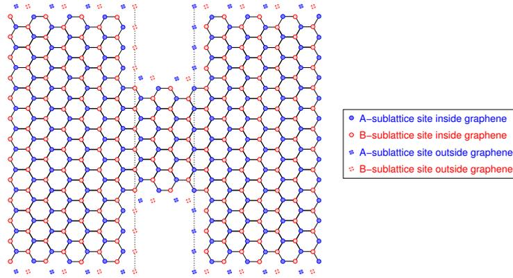
Fig. 1. Schematic representation of the graphene lattice in the presence of width discontinuities.
