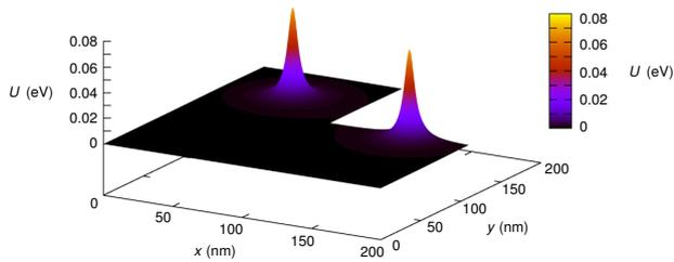
Fig. 2. Graphene structure with a width discontinuity, in the presence of a potential given by the sum of two Lorentzian functions with half-width at half-maximum 4 nm and peak height 70 meV.
