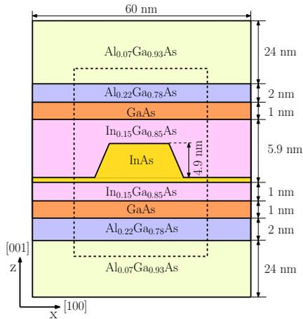
Fig. 1: Quantum dot structure. The dashed box corresponds to the electronic domain on which Schrödinger's equation is solved.
