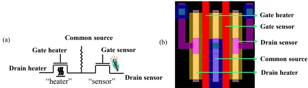
Fig. 1. (a) Two nFETs have common source connecting, can operate in a saturation and subthreshold, respectively. The structure exists for varying gate lengths and device to device pitches. (b) Mask image indicating both FETs being located in a common active area, spaced by only one poly pitch.
