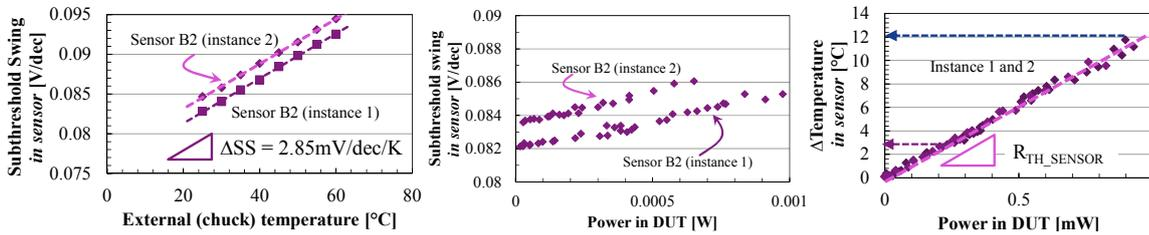
Fig. 2. Results for two instances of a device (Fig 1). (a) The subthreshold swing (SS) varies linearly with the externally applied chuck temperature. (b) When drawing a large current through the heater, the SS of the sensor varies linearly. (c) Using the initial SS as a reference, the extracted  $\Delta T$  in the sensor gives consistent results for both instances.
