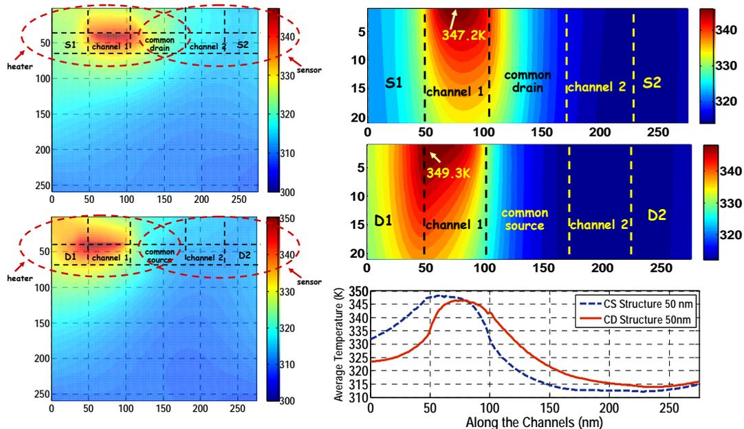
Fig. 3. Left: Lattice temperature profile for CD (top) and CS (bottom) configurations. Right: Lattice temperature profile in the active silicon layer for the two simulated structures. Average lattice temperature profile in the active silicon layer (bottom right). Multi-scale approach has been used in obtaining these results. The complete circuitry was modelled using COMSOL simulations and the boundary conditions for the active devices region was used in the thermal Monte Carlo device solver.
