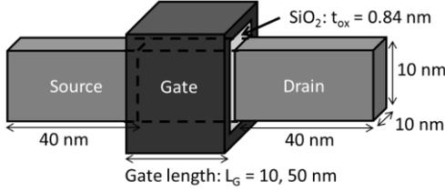
Fig. 1. Schematic of employed JL-FET structure. Donor concentration in nanowire is  $10^{19} \text{ cm}^{-3}$ .
