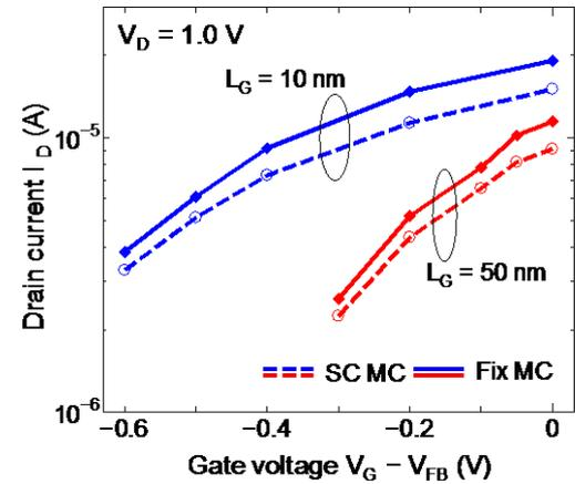
Fig. 6. Drain currents as a function of the gate voltage from SC MC and Fix MC.
