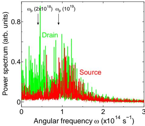
Fig. 3. Spatially averaged power spectra of potential fluctuations in the source and drain regions.  $\omega_p(2 \times 10^{18})$  and  $\omega_p(10^{19})$  are the plasma frequencies of electron density of  $2 \times 10^{18}$  and  $10^{19} \text{ cm}^{-3}$ , respectively under the same bias condition and structure used in Fig. 2.
