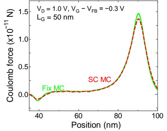
Fig. 4. Time-averaged Coulomb force of JL-FET with  $L_G = 50 \text{ nm}$  along the source-channel-drain direction from the self-consistent MC (SC MC) and the MC which turns off the long-range interaction (Fix MC) with the gate voltage of  $V_G - V_{FB} = -0.3 \text{ V}$  and the drain voltage of  $V_D = 1.0 \text{ V}$ . The gate locates from 40 nm to 90 nm.
