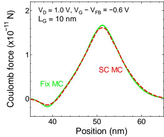
Fig. 5. Time-averaged Coulomb force of JL-FET with  $L_G = 10 \text{ nm}$  along the source-channel-drain direction with the gate voltage of  $V_G - V_{FB} = -0.6 \text{ V}$  and the drain voltage of  $V_D = 1.0 \text{ V}$ . The gate locates from 40 nm to 50 nm.
