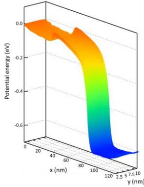
Fig. 2. Time-averaged potential profile of JL-FET with the gate length of 50 nm in the middle of nanowire cross-section under the bias condition with the gate voltage of  $V_G - V_{FB} = -0.3 \text{ V}$  and the drain voltage of  $V_D = 0.6 \text{ V}$  where  $V_{FB}$  is the flat band voltage.
