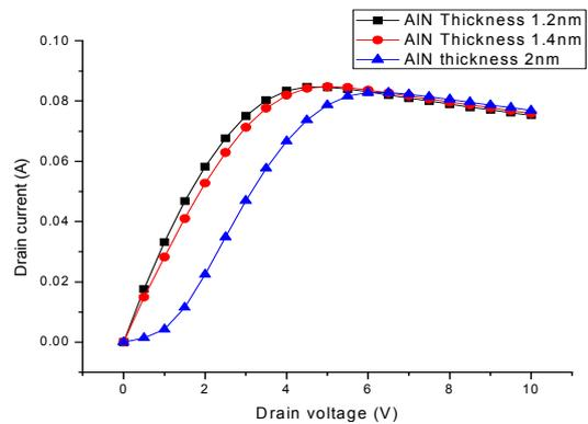
Fig. 7. The drain current versus the drain voltage, where three different AlN thicknesses are simulated.
