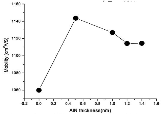
Fig. 5. The mobility versus the AlN thickness.
