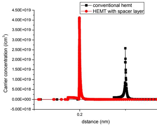
Fig. 2. The electron concentration for the device with and without AlN spacer layers.
