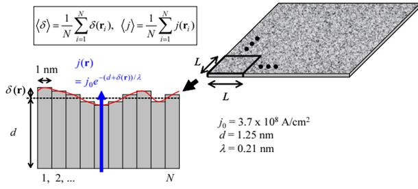
Fig. 2. Calculation method for the distribution of the tunneling current through the samples. (a) The samples with an area of  $A = L^2$  are cut out from the generated roughness pattern, and (b) in each sample the average roughness height  $\langle \delta \rangle$  and the average current density  $\langle j \rangle$  are evaluated by discretizing the sample area into small sections ( $\ll \Lambda^2$ ).
