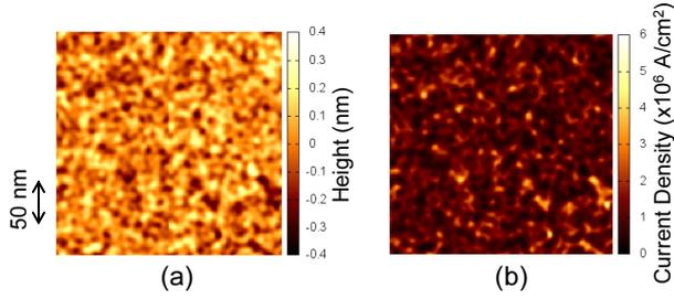
Fig. 1. Roughness pattern generated with a Gaussian spectral density  $S(q) = \pi \Delta^2 \Lambda^2 \exp(-q^2 \Lambda^2 / 4)$  ( $\Delta = 0.1$  nm,  $\Lambda = 6$  nm). (a) Distribution of the roughness height  $\delta(\mathbf{r})$  and (b) the local current density  $j(\mathbf{r})$  are plotted.
