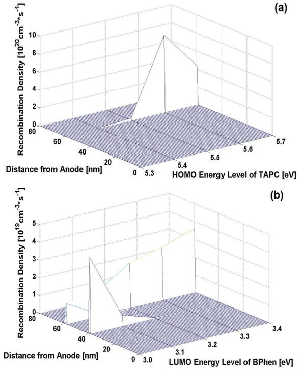
**Fig. 3.** (a) Recombination density profile for different HOMO energy level of TAPC [eV].
