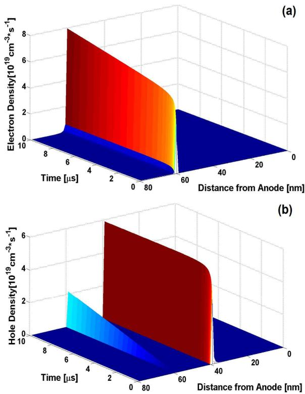
**Fig. 2.** (a) Calculated electron density profile in OLED after turn-on [10μs]
