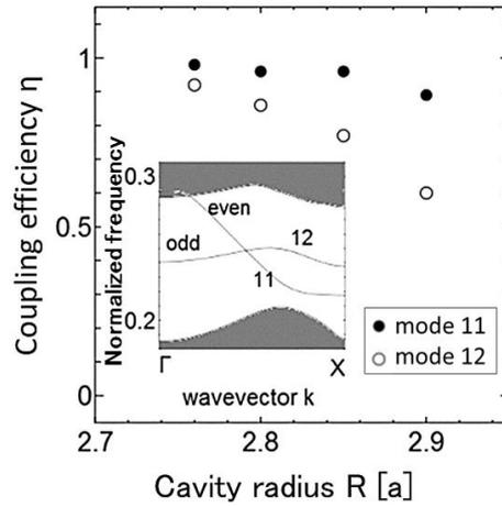
Fig. 3. Coupling efficiency of cavity radius  $R=2.76a$ ,  $2.80a$ ,  $2.85a$ , and  $2.90a$ . Filled circles and open circles denote the coupling efficiency related to the mode 11 and 12. Inset: Photonic band diagram. The curves labeled as 11 and 12 are waveguide modes.
