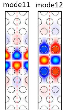
Fig. 4. Calculated magnetic field amplitude of mode 11 (left) and 12 (right) for wave vector  $X$ . Mode 11 and 12 have even and odd symmetry, respectively with respect to the center of the WGM (red dash line).
