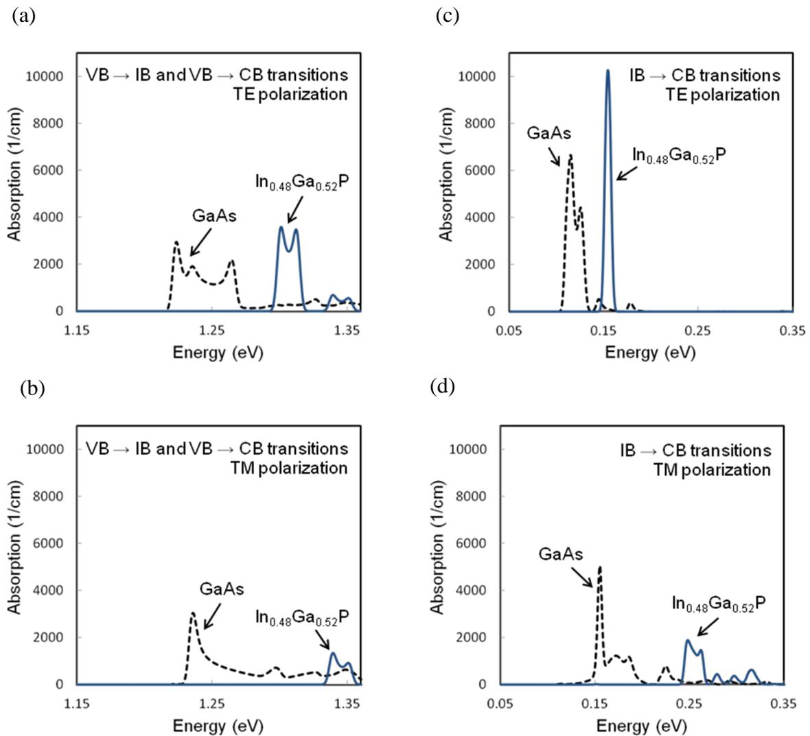
Fig. 2. The absorption spectra of InAs/GaAs QDSLs (dashed line) and InAs/ $In_{0.48}Ga_{0.52}P$  QDSLs (solid line) (a) TE polarized in the  $VB \rightarrow IB (MB_0)$  and  $VB \rightarrow CB$  transitions, (b) TM polarized in the  $VB \rightarrow IB (MB_0)$  and  $VB \rightarrow CB$  transitions, (c) TE polarized in the  $IB (MB_0) \rightarrow CB$  transitions, and (d) TM polarized in the  $IB (MB_0) \rightarrow CB$  transitions.
