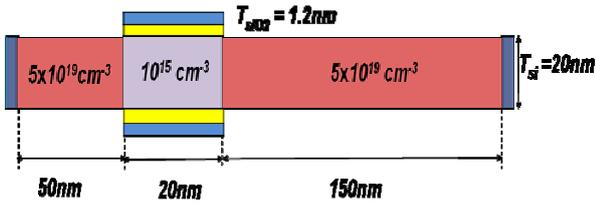
Fig. 1. Simulated Double-Gate MOSFET.
