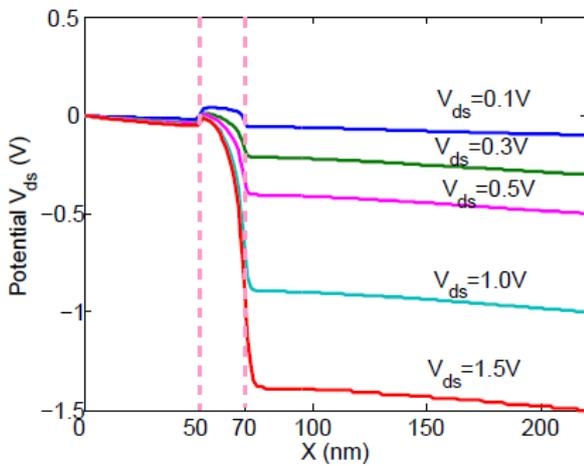
Fig. 2. Potential profile (bottom of conduction band) for various  $V_{DS}$  at  $V_G = 0.5$  V (isothermal simulations).
