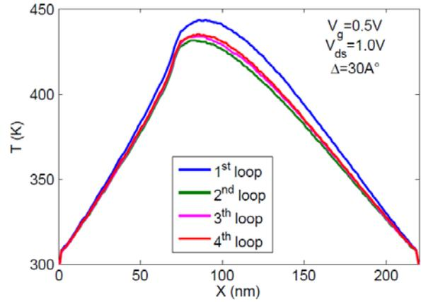
Fig. 4. Profile of effective temperature  $T_{eff}$  along the device obtained at a given bias point after different loop numbers.
