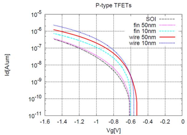
Fig. 5.  $I_{ds}$ - $V_g$  characteristics predicted by the present model. Scaling merit is observed stronger in wire-TFETs.
