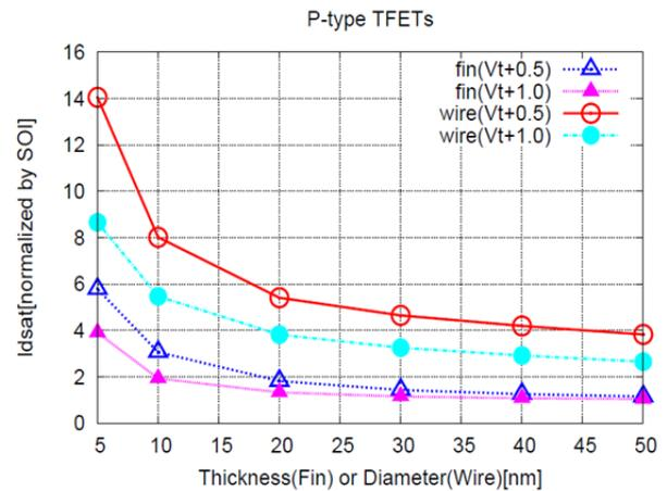
Fig. 6. Size scaling merits of saturation current at  $V_g = V_t - 0.5, V_t - 1.0$  ( $V_t @ I_{ds} = 10^{-11}$  [A/ $\mu\text{m}$ ]) of fin and wire-type TFETs. Currents are normalized by those of SOI-TFETs.
