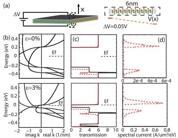
Fig. 3. Transport simulation for SmSe with hydrostatic strain. (a) Device configuration and supercell of simulation domain. (b) Real and imaginary band structure for 0% and 3% hydrostatic strain. (c) Transmission with 0V and 0.05V linear drop potential. (d)  $V_d=0.05\text{V}$ , spectral current with linear drop potential.
