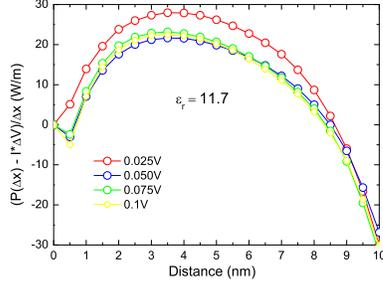
Fig. 3. Spatial distribution of the difference between equation (9) and its non-interacting limit (11) for an homogenous dielectric permittivity. The active region has been split up into 20 infinit contiguous volumes  $\Omega$ . Carrier “bunching” causes a positive difference between the exact value of the electric power spatial density and its non-interacting limit  $\langle I \rangle \cdot \langle \Delta V \rangle$  value. The contrary happens in presence of “antibunching” of carriers.
