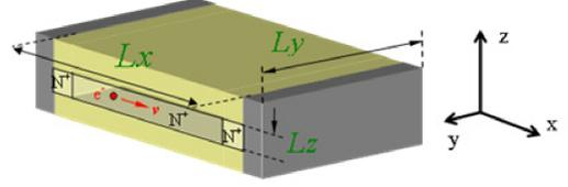
Fig. 1. Schematic picture of the simulated Silicon  $N^+NN^+$  resistor.  $N^+ = 6.25E18$ ,  $L_x = 10nm$ ,  $L_y = 30nm$ ,  $L_z = 30nm$ .  $N$  refers intrinsic Silicon.
