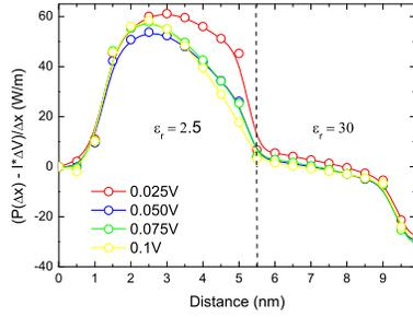
Fig. 4. Spatial distribution of the difference between equation (9) and its non-interacting limit (11) for bipartite dielectric permittivity. The manipulation of the active region electrostatic parameters can be designed to increase bunching and antibunching dynamics. The discrepancy between the kinetic energy gain rate and  $\langle I \rangle \cdot \langle \Delta V \rangle$  can be then stressed.
