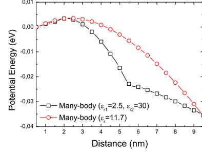
Fig. 5. The manipulation of the active region dielectric permittivity induces a change on the average conduction band distribution that modifies the way carriers interact with each other.
