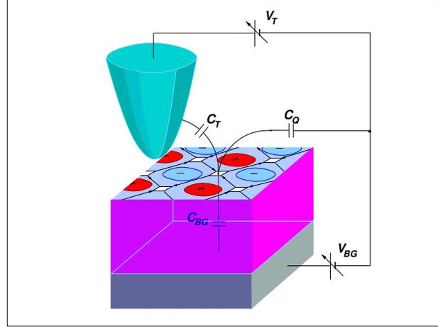
Fig. 3. Illustration of the model used to establish a link of the random network model with some of the parameters that can be tuned in the setup of a scanning gate spectroscopy experiment.  $C_Q$  is the quantum capacitance (per unit area) at the considered saddle point.
