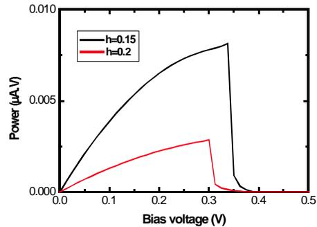
Fig. 6. Left electrical power as a function of the bias voltage
