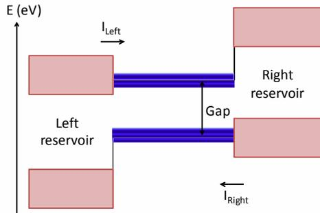
Fig. 2. Band diagram of the quantum wire-dot-wire junction
