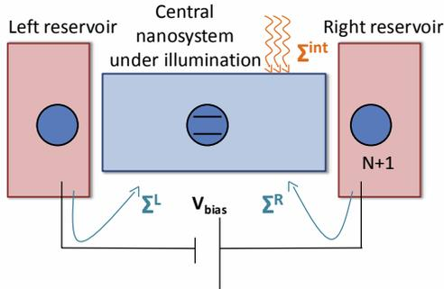
Fig. 1. Modeling of the quantum wire-dot-wire junction
