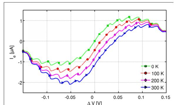
Fig. 2. Electronic current as a function of bias voltage for different temperature gradients between the contacts.
