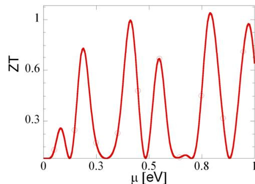
Fig. 3. Thermoelectric factor ZT as a function of the chemical potential  $\mu$  at room temperature.
