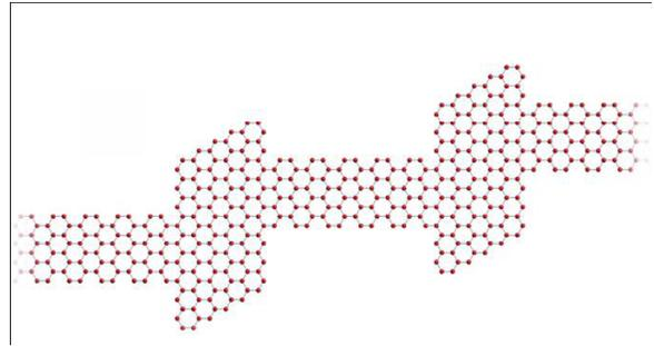
Fig. 1 Mixed GNR structure optimized to provide high ZT.
