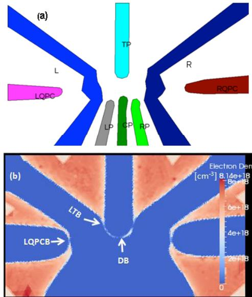
Fig.1. (a) Top view of the depletion gate pattern in a 3D Si quantum dot. (b) Top view of electron density at the Si/SiO<sub>2</sub> interface and T = 0.2 K. The gate voltages that meet the optimization targets are AG = 3.48 V, TP = -0.74 V, CP = -0.007 V, LP = RP = -5.95 V, L = R = -1.15 V, LQPC = RQPC = -2.41 V.
