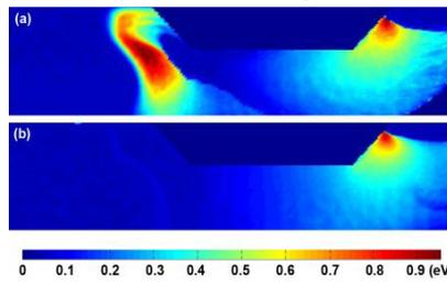
Fig. 5 Average electron energy distribution in the Si film at (a)  $V_{gs}=0, V_{ds}=55V$ , and (b)  $V_{gs}=5.0V, V_{ds}=40V$ , respectively.
