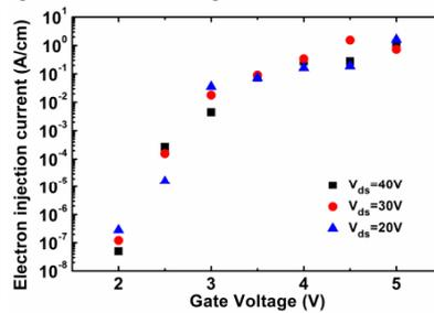
Fig. 10 Total electron injection current into oxide. Larger gate voltage induces larger electron injection current, while the drain bias has rare influence on the oxide injection current.
