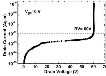
Fig. 2 Drain breakdown characteristics of the LDMOS transistor. The BV is defined as the drain voltage at which the drain current exceeds 1pA/μm at  $V_{gs}=0V$ .
