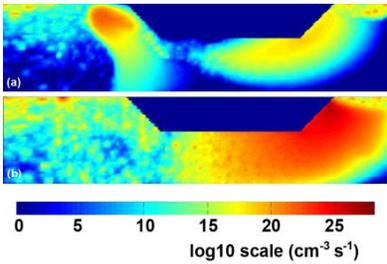
Fig. 7 II rate distribution in the Si film at (a)  $V_{gs}=0, V_{ds}=55V$ , and (b)  $V_{gs}=5.0V, V_{ds}=40V$ , respectively.
