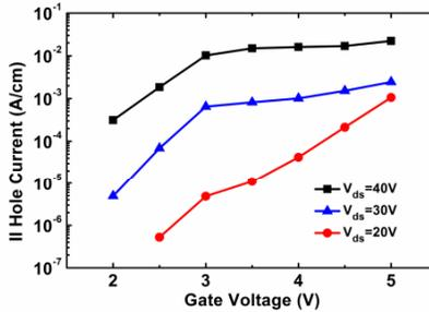
Fig. 8 Total II generated hole current under different bias conditions. The II hole current increases rapidly with the increase of the gate and drain voltage.
