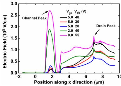
Fig. 4 Electric field in the Si film along the dashed line in Fig. 1 under various gate and drain biases, of which two peaks can be observed.
