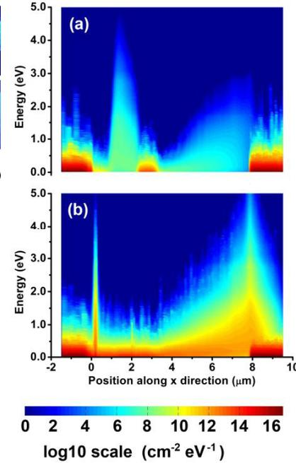
Fig. 6 Energy resolved electron distribution function in the Si film at (a)  $V_{gs}=0, V_{ds}=55V$ , and (b)  $V_{gs}=5.0V, V_{ds}=40V$ , respectively.
