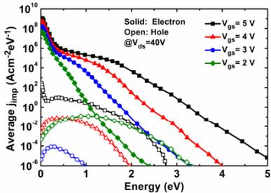
Fig. 9 Energy distribution of the gate average impingement current density induced by carriers in the channel hitting the gate oxide at  $V_{ds}=40V$  and different  $V_{gs}$ .
