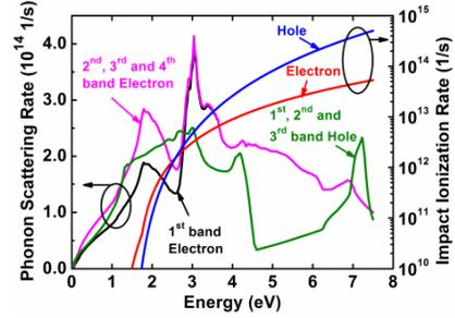
Fig. 3 Phonon scattering and II rates versus energy for different electron and hole bands.
