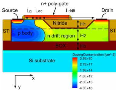
Fig. 1 The SOI LDMOS device structure studied in this work. Colours indicate the realistic doping profile of the device.
