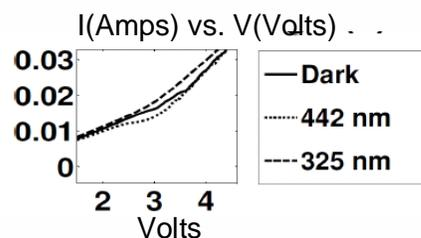
Fig. 4. I-V characteristics of MEH-PPV/CdSe system at room temperature.
