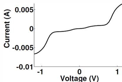
Fig. 3. I-V characteristics simulated on a single quantum dot between two metal electrodes; the case illustrated is for P3HT/CdSe DBQWD energy levels 0.13 eV and 0.45 eV. Extended results will be presented/
