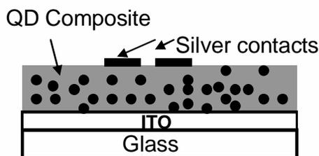
Fig. 1. Generic QD nanocomposite structure considered in this modeling effort.
