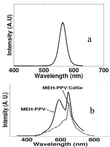
Fig. 2. (a) PL of CdSe (b) PL of MEH-PPV/CdSe system comparing with PL of MEH-PPV. The EA values of CdSe QDs, MEH-PPV and P3HT is 3.7 eV, 2.8 eV and 3.2 eV.  $U_{POL-MEH-PPV}$  is 0.2 eV and  $U_{POL-P3HT}$  is 0.5 eV. Thus, electron transport is possible from MEH-PPV and P3HT to CdSe QDs. This is consistent with the observed quenching of the PL peaks from the polymers.
