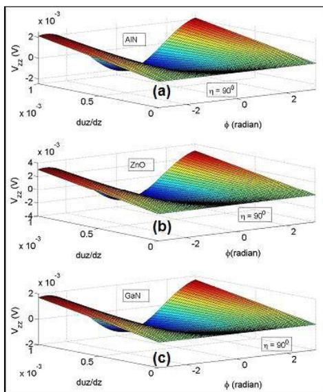
Fig. 2. Piezoelectric potential distribution for phonon propagation at an angle  $\eta = 90^\circ$  for zincblende structures.
