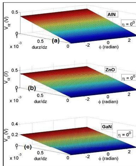
Fig. 3. Piezoelectric potential distribution for phonon propagation at an angle  $\eta = 0^\circ$  for wurtzite structures.
