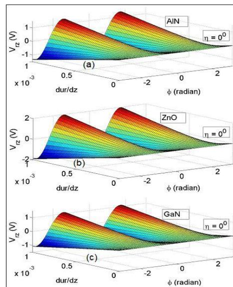
Fig. 4. Piezoelectric potential distribution for phonon propagation at an angle  $\eta = 0^\circ$  for zincblende structures.
