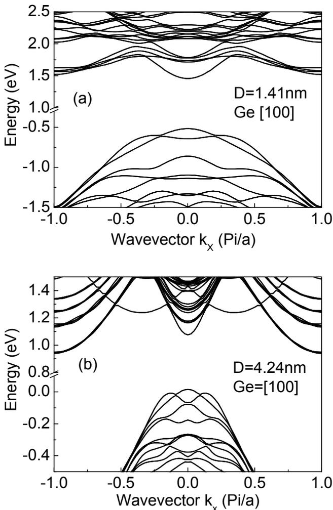
Fig. 2. Energy bandstructures of [100]-oriented Ge nanowires with two diameters: a) 1.41 nm and b) 4.24 nm. The transverse surfaces are {100} faces with dangling bonds pacified by hydrogen. The lattice constant  $a=0.5658$  nm and  $k_x$  is the wavevector along the nanowire axis.
