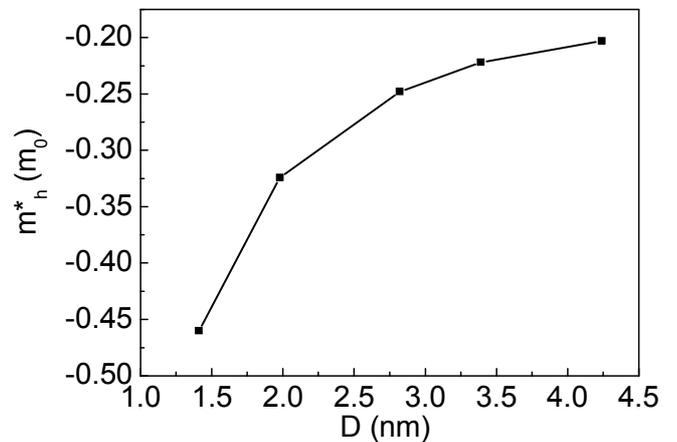
Fig. 4. Hole effective mass  $m_{*h}^*$  at the  $\Gamma$  point in the valence band versus the wire diameter  $D$  for a [100]-oriented Ge nanowire.  $m_0$  is the free electron mass.
