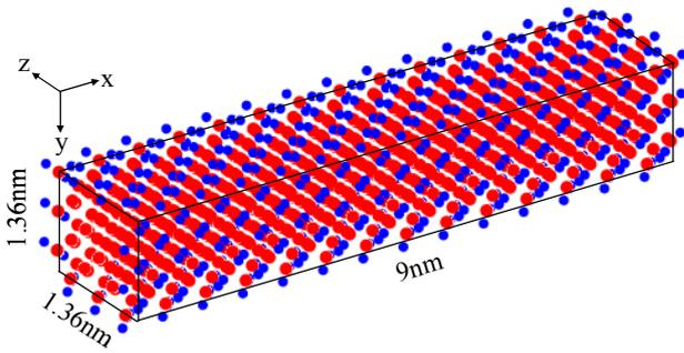
Fig. 1. Atomistic view of a Ge square nanowire [1.36nm  $\times$  1.36nm  $\times$  9nm] playing the role of the conduction channel in the active region of the transistor. Germanium atoms are in red and the dangling bonds are saturated by hydrogen atoms (in blue).
