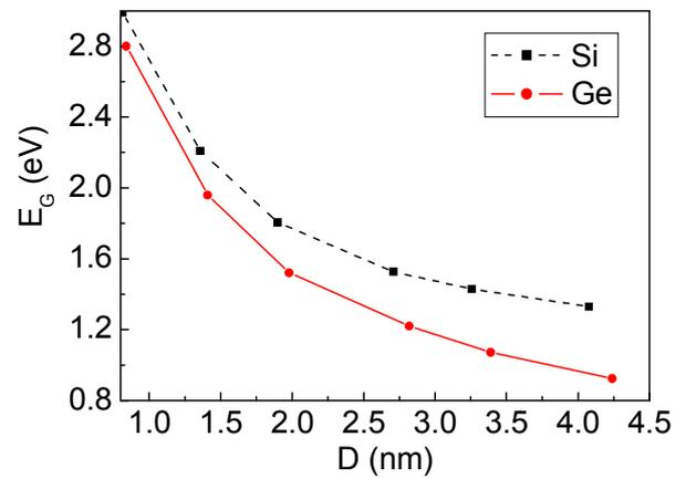
Fig. 3. Bandgap versus the diameter  $D$  of Ge and Si [2] nanowires with axis oriented along the [100] direction. The same surface configuration (orientation and boundary conditions) is considered for the both materials.
