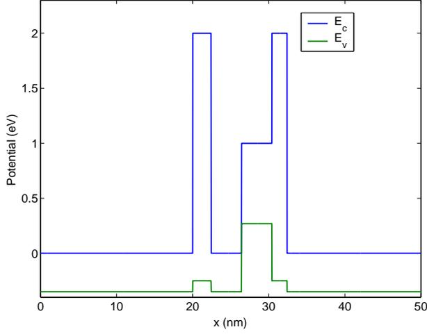
Fig. 1. Band alignments of the double barrier structure used in the simulations.
