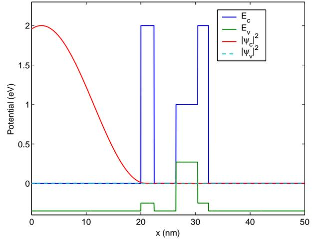
Fig. 4. Conduction and valence envelope functions,  $\psi_c$  and  $\psi_v$ , related to the resonant energy  $E = 1.18$  eV for the spin-down case.
