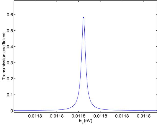
Fig. 2. Transmission coefficient spectra for the *InAs/GaSb/AlSb* diode of Fig. 1 related to the spin up conduction electrons.
