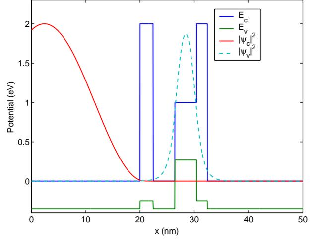
Fig. 3. Conduction and valence envelope functions,  $\psi_c$  and  $\psi_v$ , related to the resonant energy  $E = 1.18$  eV for the spin-up case.
