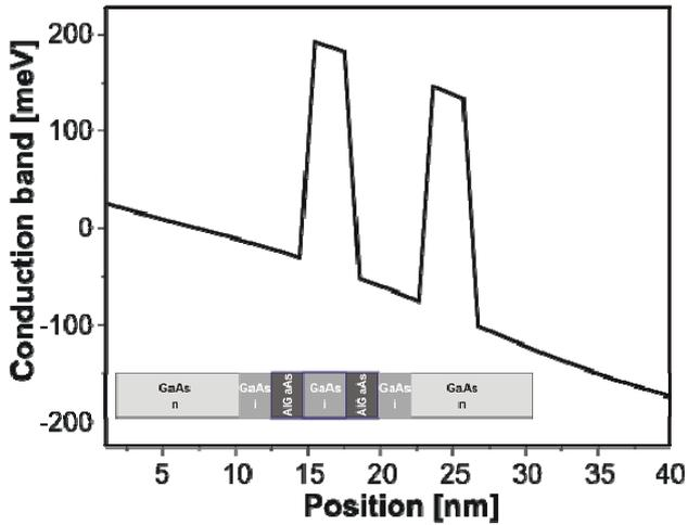
Fig. 1. Conduction band energy of the GaAs/Al<sub>3</sub>Ga<sub>7</sub>As resonant tunneling structure described in the text, at a bias voltage of 200 mV.
