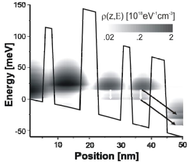
Fig. 3. Potential profile of 50 nm GaAs/Al<sub>15</sub>Ga<sub>85</sub>As quantum cascade laser structure from Ref. [4] at a bias voltage of 60 mV. The energy resolved electron density is shown as contour plot. The arrows are only meant to guide the eye and show the calculated emission energies (white = photons, black = phonons).
