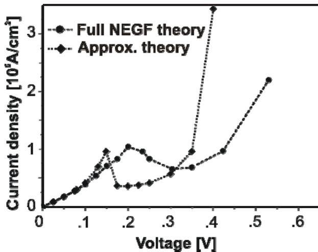
Fig 2. Calculated current density in the GaAs/Al<sub>3</sub>Ga<sub>7</sub>As resonant tunneling structure of Fig. 1 with (circles) and without (diamonds) off-diagonal inelastic scattering. The connecting lines are only meant to guide the eye.
