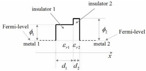
Fig. 1. Potential profile of the double-insulator-layer MIM diode without applied voltage
