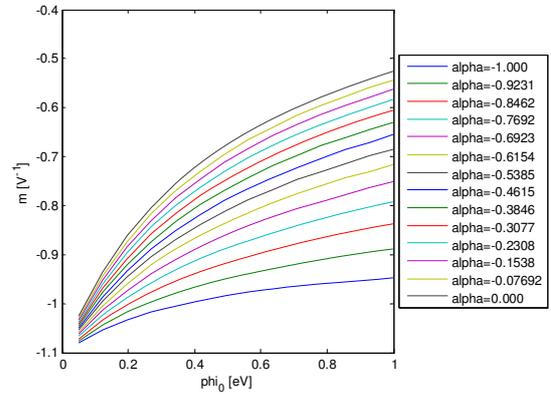
Fig. 5.  $m$  as a function of the average work function  $\phi_0$  and the  $\alpha$  asymmetry factor of the work functions
