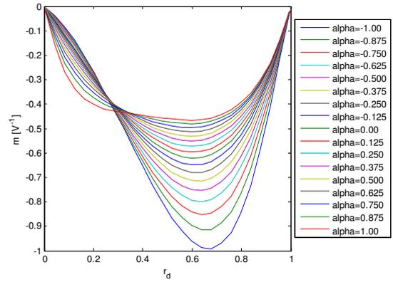
Fig. 4.  $m$  as a function of the thickness ratio  $r_d$  and the  $\alpha$  asymmetry factor of the work functions
