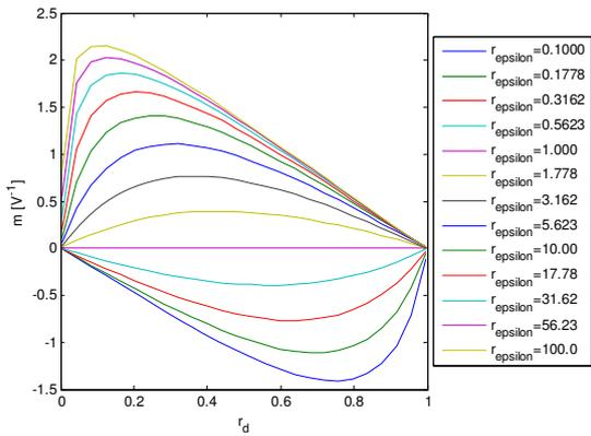
Fig. 3.  $m$  as a function of the thickness ratio  $r_d$  and the dielectric constant ratio  $r_\epsilon$
