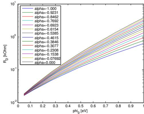
Fig. 6.  $R_D$  as a function of the average work function  $\phi_0$  and the  $\alpha$  asymmetry factor of the work functions
