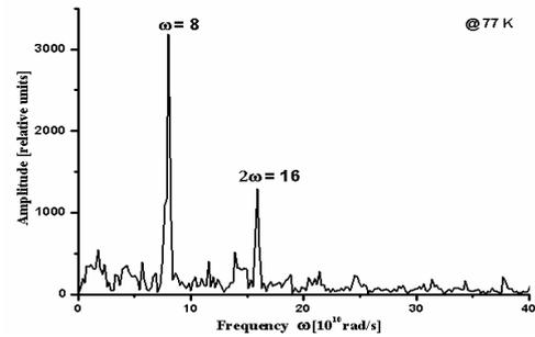
Fig. 3. Spectral components of the electric field of space charge wave at the output antenna with an excitation input signal ( $\omega = 8 \times 10^{10}$  rad/s) at 77 K.
