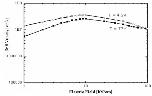
Fig. 2. Steady-state drift velocity as a function of electric field in strained Si/SiGe heterostructure at 4.2 and 77 K.
