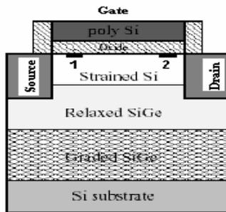
Fig. 1. Cross-section of the strained Si/SiGe heterostructure, 1 and 2 are input and output antenna respectively.
