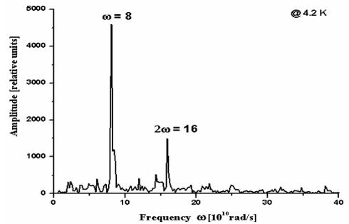
Fig. 4. Spectral components of the electric field of space charge wave at the output antenna with an excitation input signal ( $\omega = 8 \times 10^{10}$  rad/s) at 4.2 K.
