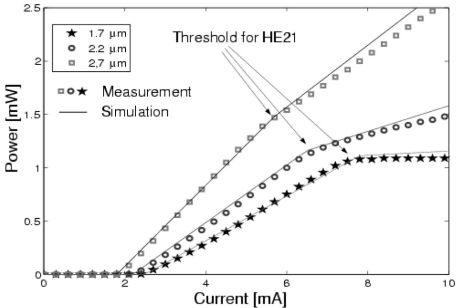
Fig. 2. Simulated (solid lines) and measured power-current characteristics of VCSEL designs with different metal aperture radii at  $T = 303 \text{ K}$ . With decreasing metal aperture, the threshold currents for the fundamental and higher order modes increase due the higher absorption in the metal. Concurrently, the slope efficiency decreases since the power generated in the device is absorbed in the metal, too.
