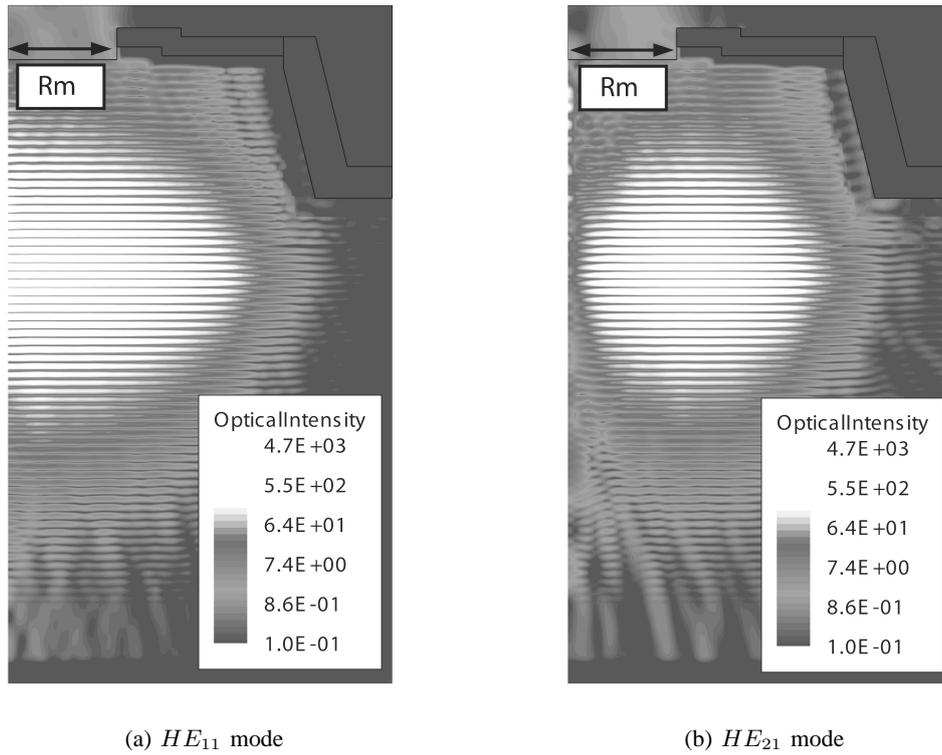
Fig. 1. Normalized optical intensity for a VCSEL with metal aperture radius  $R_m < 3.5 \mu\text{m}$ . Due to absorption in the metal, the total losses for the  $HE_{21}$  mode are significantly higher than for the fundamental  $HE_{11}$  mode. This results in an improved single-mode behaviour.
