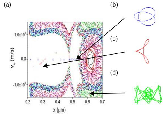
**Fig. 3.** (a) Poincaré section at the MR peak. (b) A periodic orbit (blue open symbols), (c) backscattered trajectory (red open symbols) (d) chaotic trajectory (green points). The arrows mark points representing  $v_x$  and  $x$  at  $y=0$  on the trajectories shown.
