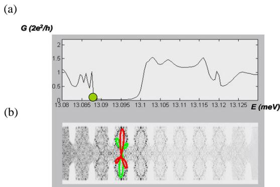
**Fig. 2** (a) The calculated conductance as a function of energy at the magnetic field position above the MR peak. The green point indicates the energy position for the calculated  $|\psi(x,y)|^2$ . (b) The  $|\psi(x,y)|^2$  in the 3<sup>rd</sup> resembles two *closed* trajectories (red and green) that are classically inaccessible from the outside, indicating that conductance is only possible by assuming phase space tunnelling.
