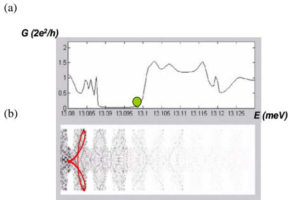
**Fig. 1.** (a) The calculated conductance as a function of energy at the magnetic field position of the MR peak. The Green point indicates the energy position for the calculated  $|\psi(x,y)|^2$ . (b)  $|\psi(x,y)|^2$  looks like an *open, backscattered* trajectory of the classical calculation (superimposed in red in the 1st dot).
