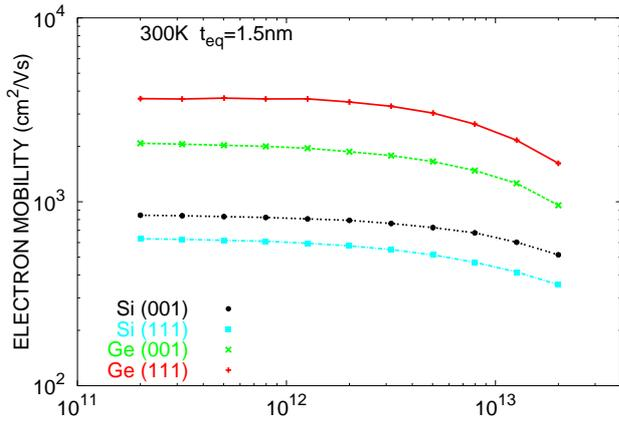
Fig. 1. Calculated phonon limited electron mobility in Si and Ge inversion layers as a function of electron sheet density.
