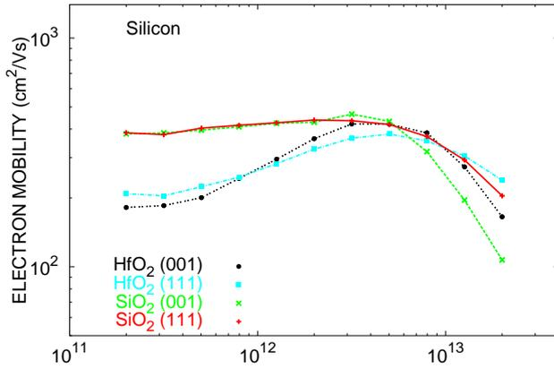
Fig. 2. Total calculated mobility, including scattering with bulk phonons, surface roughness and high- $\kappa$  phonons (Si only), as a function of electron sheet density.
