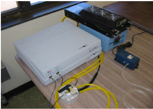
Fig. 1. The experimental I(T) modeling system incorporates a computer-controlled pulsed I-V instrument and thermal chuck.
