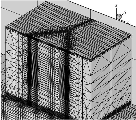
Fig. 2. Detail of a gate meshed for the simulation of three grains in polysilicon.
