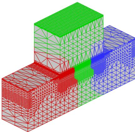
Fig. 3. Partition of the finite element mesh in three subdomains.
