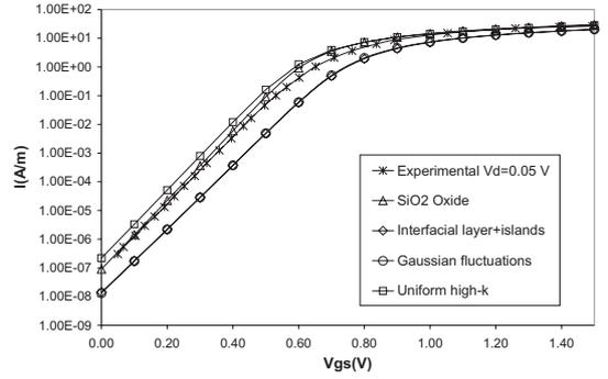
Fig. 4.  $I_D - V_G$  characteristics obtained from the 3D D-D parallel simulator compared with experimental data for the 67 nm effective gate length Si MOSFET.
