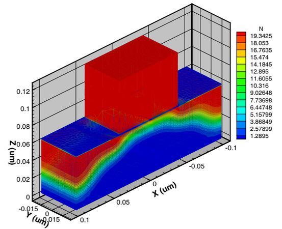
Fig. 5. Electron density on log scale in the 67 nm effective gate length Si MOSFET at  $V_G = 0.5V$  and  $V_D = 0.05V$ .
