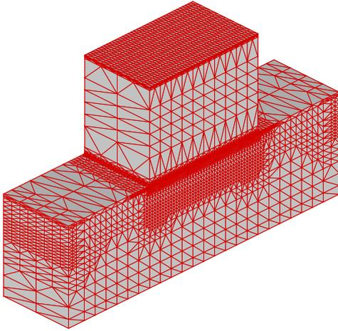
Fig. 1. Finite element mesh for simulation of the 67 nm effective gate length Si MOSFET with a polysilicon gate.
