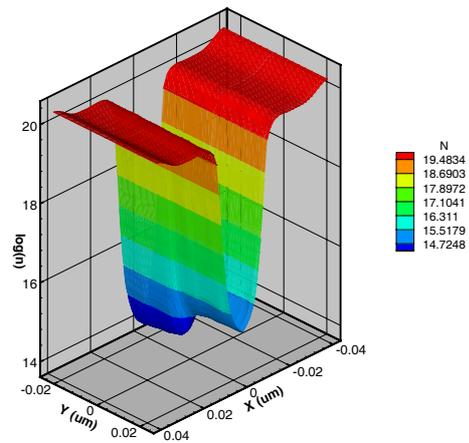
Fig. 6. Electron density at equilibrium beneath a dielectric layer with two different dielectric constants of 7 ( $Si_3N_4$ ) and 5 in the template 25 nm gate length bulk MOSFET.
