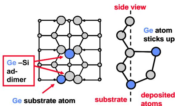
Fig. 3 Illustration of the surface dimer exchange mechanism. When two Ge adatoms meet on the surface, they form a dimer. However, it then becomes energetically favorable for one Ge atom to exchange places with a Si atom in the the substrate, resulting in a mixed dimer on the surface.
