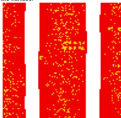
Fig. 6 The fourth atomic layer after deposition, with red corresponding to where there are Ge atoms and orange to Si. The Si atoms have been promoted from the substrate mainly via the exchange mechanism illustrated in Fig. 3.
