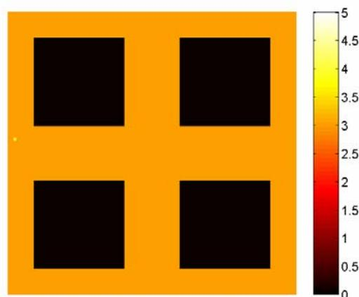
Fig. 4 The Si surface after a single Ge adatom has been deposited. Color indicates the number of atomic layers. The initial substrate has been patterned so that there is a Si grid, three atomic layers high and square voids.
