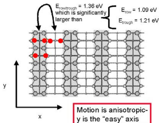
Fig. 2 The A top view of the reconstructed Si (100) surface. The diffusion of adatoms and ad-dimers across the reconstructed surface is anisotropic, with activation energies depending on whether the diffusion is  $\perp$  or  $\parallel$  to the dimer rows.
