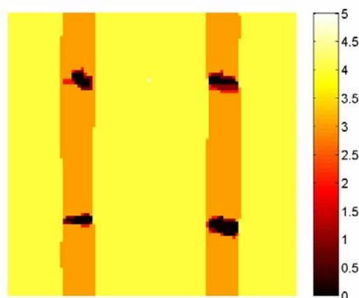
Fig. 5 As above, but after after two monolayers of Ge have been deposited at 470 K. The initial grid combined with the anisotropic hopping barriers have led to the formation of Ge/Si stripes on the surface.
