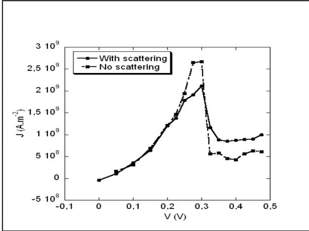
Fig. 1. J/V characteristic of a 300K GaAs RTD, with scattering activated and deactivated
