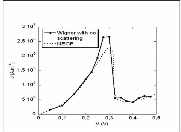
Fig. 4. Comparison of the characteristic of the RTD with scattering deactivated with a fully self-consistent ballistic NEGF calculation
