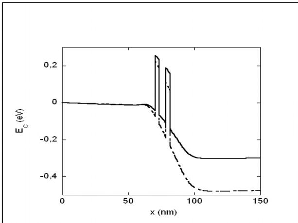
Fig. 3 Self-Consistent potential profiles of the RTD for  $V=0.3$  (plain line) and  $V=0.475V$  (dotted line)
