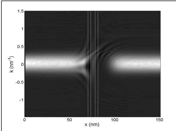
Fig. 2. Wigner function for an on-resonant state ( $V=0.3V$ )
