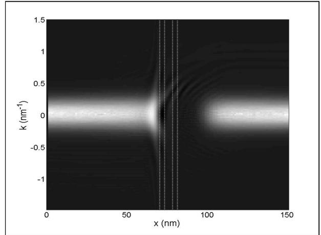
Fig. 5. Wigner function for an off-resonant state ( $V=0.475V$ )
