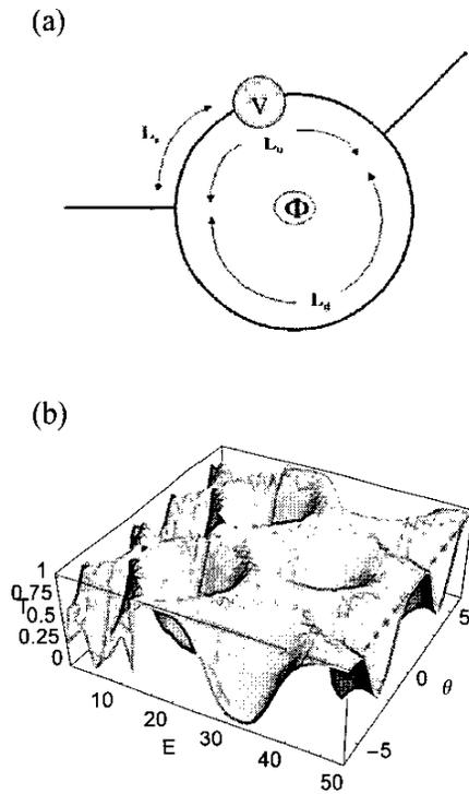
**Fig. 2.** (a) Geometry of an asymmetric ring with an attractive potential dot. The lengths of upper and lower arms are  $L_u$  and  $L_d$  correspondingly, and  $L_s$  is distance of the dot from left junction. (b) 3D plot of electron transmission through the asymmetric ring, showing variation with electron energy and threaded magnetic flux.
