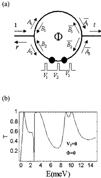
**Fig. 1.** (a) AB ring with embedded coupled QDs. The coupling of the double QDs in series can be controlled by the modulation of centered potential barrier  $V_2$ . (b) The Fano and Breit-Wigner resonances in the transmission as a function of electron energy are shown for  $V_2=0$  and  $\Phi=0$ .
