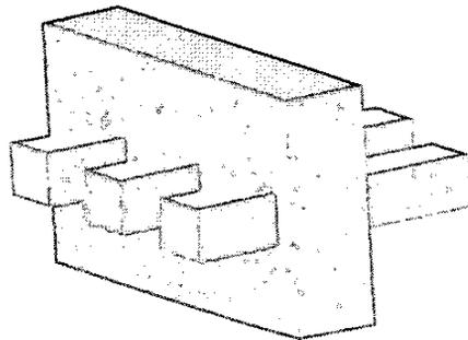
Figure 2: A 3D view of the square - shaped copper-low- $\kappa$  interconnects.
