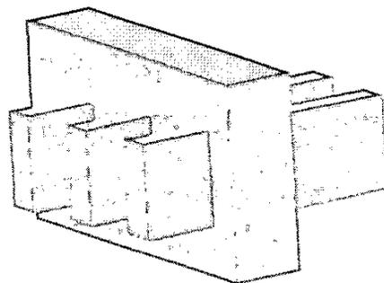
Figure 3: A 3D view of the rectangular - shaped copper-low- $\kappa$  interconnects.
