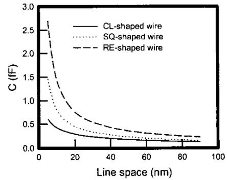
Figure 4: The calculated parasitic capacitance for the three interconnects with different line space.
