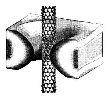
Figure 1: potential and charge density isosurfaces of a coaxially gated (10,0) semiconducting CNT in equilibrium conditions ( $V_{ds}$ =0.0V), when a potential of 0.2V is applied to the gate contact causing a local negative charge accumulation.
