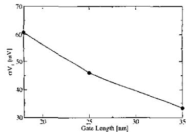
**Fig. 5**  $V_T$  variation as a function of scaled device gate length.
