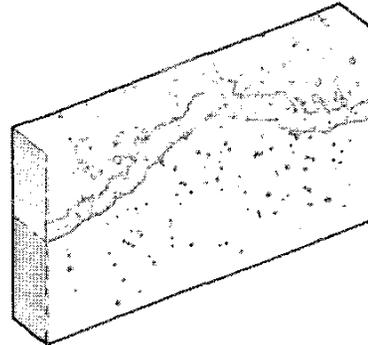
**Fig. 4** 3D-Potential distribution in a 35nm 'atomistic' device
