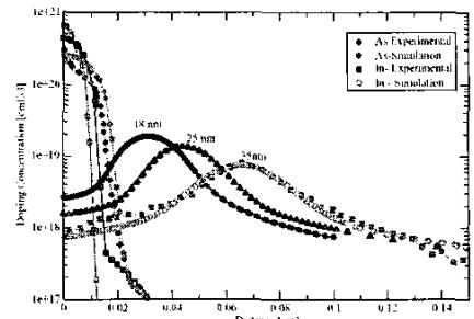
**Fig.2** 1-D Channel doping profiles of calibrated 35, 25 and 18nm scaled devices.
